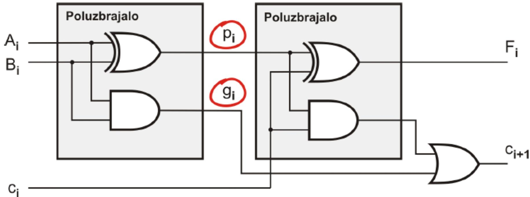
$$g_i = A_i \cdot B_i \quad \text{signal generiranja bita prijenosa}$$
