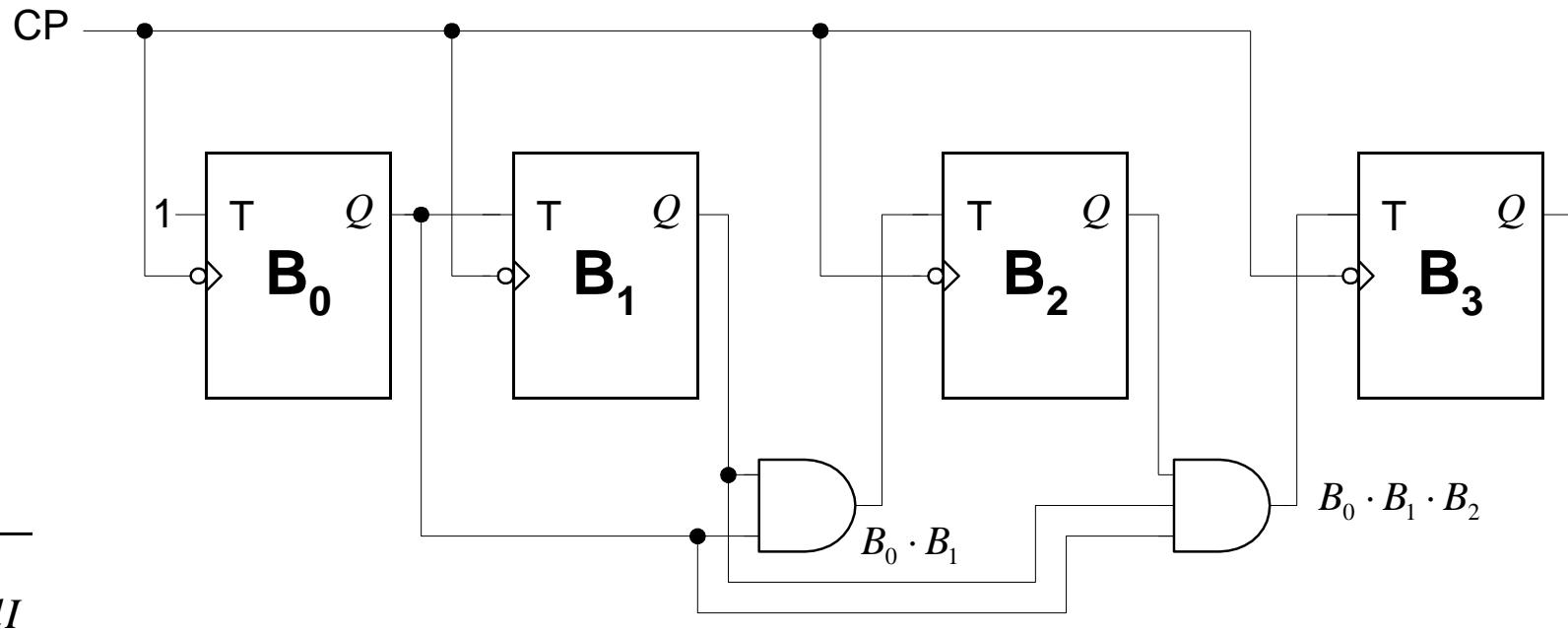
$$f_{\max} = \frac{1}{t_{\text{setup}} + t_{\text{db}} + t_{dI}}$$
