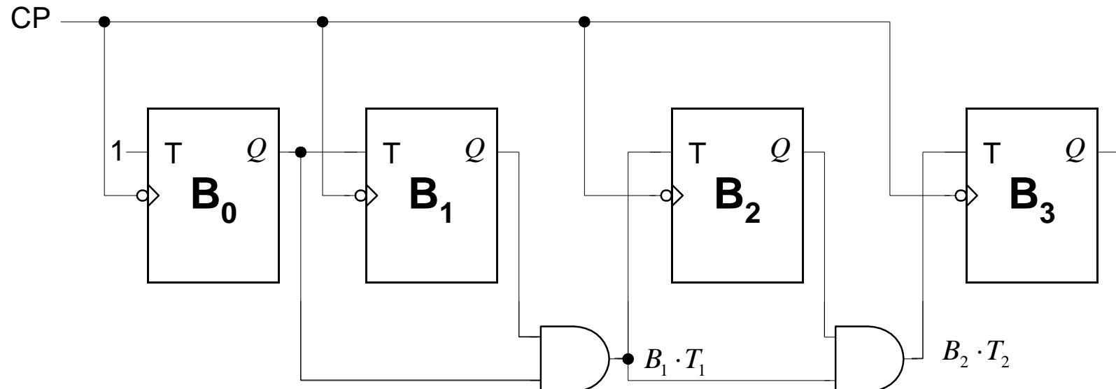
$$f_{\max} = \frac{1}{t_{\text{setup}} + t_{db} + (n-2) \cdot t_{dI}}$$
