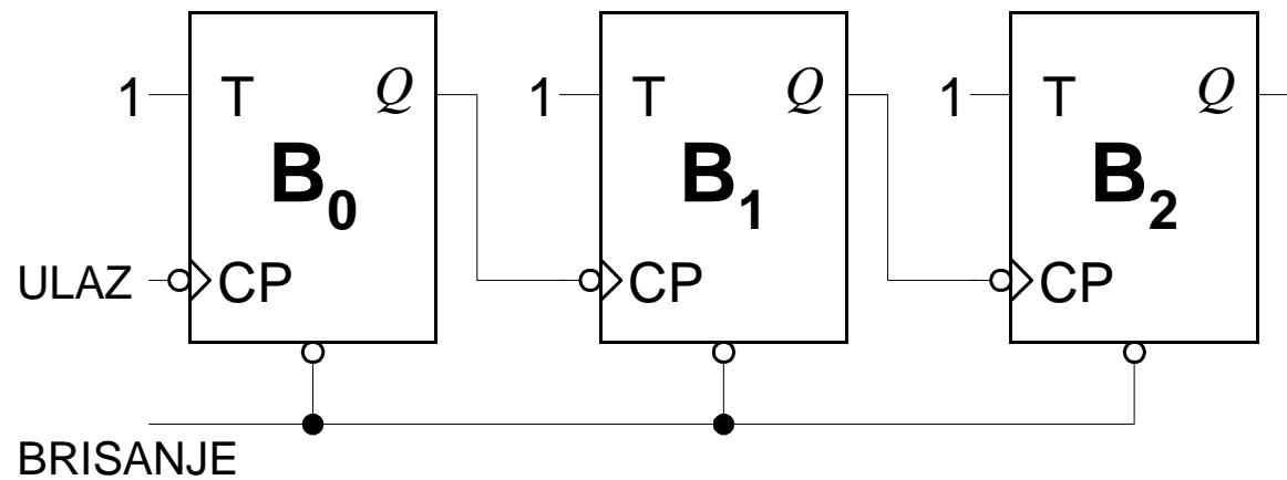
$$\begin{aligned}D_0 &= \overline{B}_2 \overline{B}_1 \overline{B}_0 \\D_1 &= \overline{B}_2 \overline{B}_1 B_0 \\&\vdots \\D_7 &= B_2 B_1 B_0\end{aligned}$$
